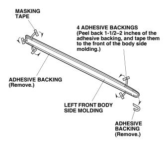
3. Using one alcohol pad, clean the door where the left front upper molding will attach.
