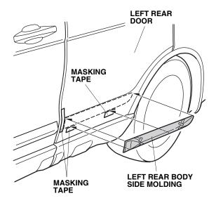
10. Position the left rear body side molding on the left rear door, aligning it with the masking tape you attached in step 7.
