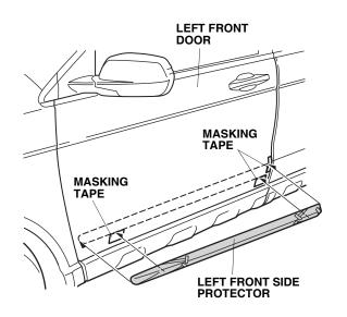
4. Position the left front molding on the left front door, aligning it with the masking tape you attached in step 1.
