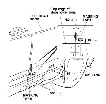
8. Peel back 1-1/2–2 inches of the adhesive backing, and tape them to the front of the rear body side molding. Remove the front and rear adhesive backings.
